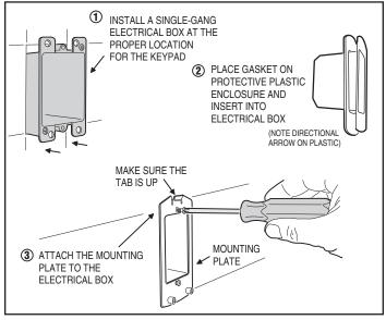
Figure 4. Installing the Mounting Plate
